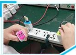
9. Aging test for travel charger
