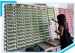
9. Aging test for travel charger
